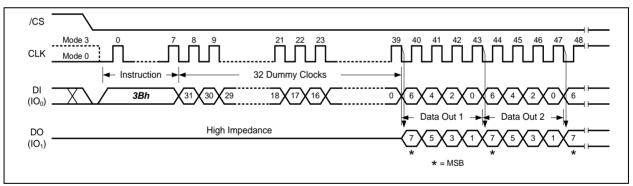
Figure 22b. Fast Read Dual Output Instruction (Continuous Read Mode, BUF=0)
