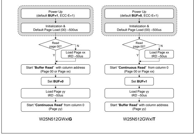
Figure 3. W25N512GW Flash Memory Operation Diagram
