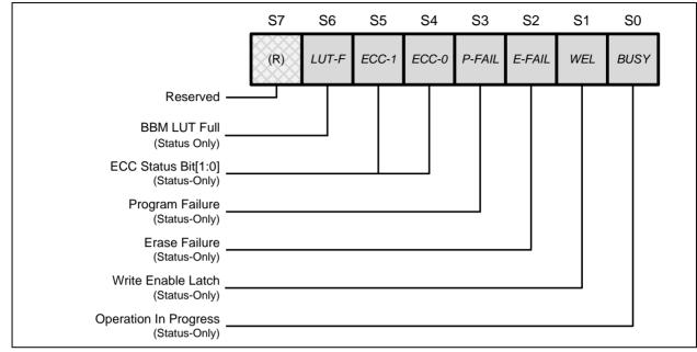
Figure 4c. Status Register-3 (Address Cxh)
