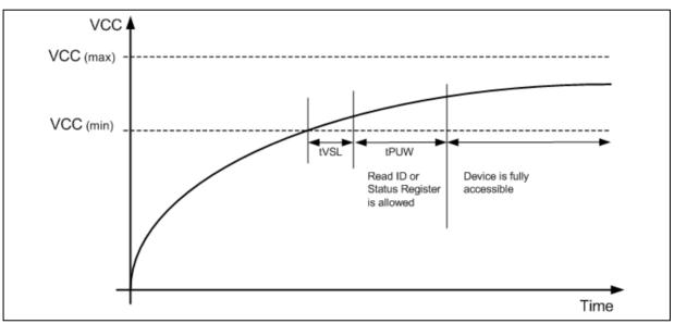
Figure 33a. Power-up Timing and Voltage Levels
