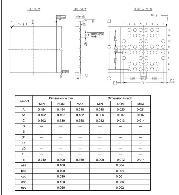
Note: Dimension b is measured at the maximum solder bump diameter, parallel to primary datum C.
