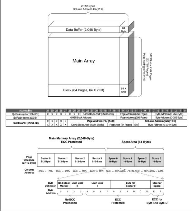
Figure 2. W25N512GW Flash Memory Architecture and Addressing
