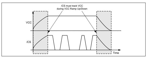
Figure 33b. Power-up, Power-Down Requirement
