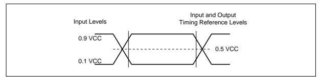
Figure 34. AC Measurement I/O Waveform
